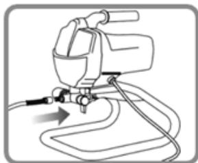
1 - FIXE A MANGUEIRA DE TINTA NA CONEXÃO DE MANGUEIRA E APERTE COM A CHAVE INGLESA PARA APERTAR
